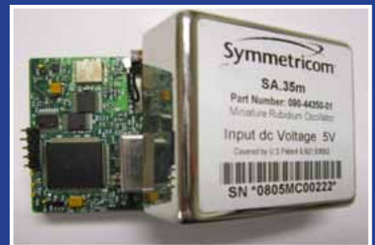
Tactical-grade Atomic Clock, volume: <math>< 3 \text{ cm}^3</math>, power: <math>< 100 \text{ mW}</math>.
